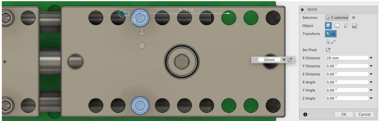
Next, locate the Test CUBE so the transparent square overlaps the gripper setscrews on the right by about 0.01". Note, when material is placed in the vise between the grippers, some of the stock material will be crushed. By overlapping material with the grippers, users will get a better representation of what is actually happening on the machine.
