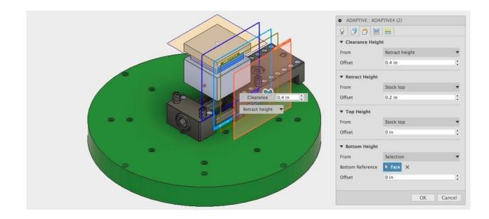
The toolpath should look like the image below. Before Posting a tool path, users should check for collisions with the Pocket NC vise using the Simulate feature within the ACTIONS dropdown.
