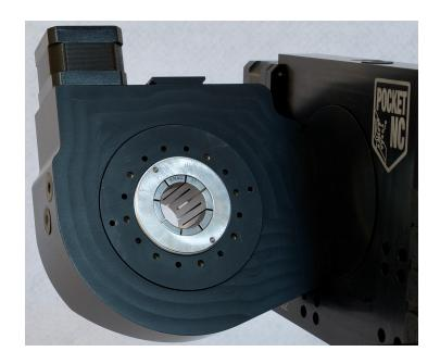
Another way that stock can be mounted on the Pocket NC V2 is using the ER-40 collet fixture. This is a particularly useful way to hold round stock, especially because the through-hole design allows the user to mount longer parts than could be held in the vise.
