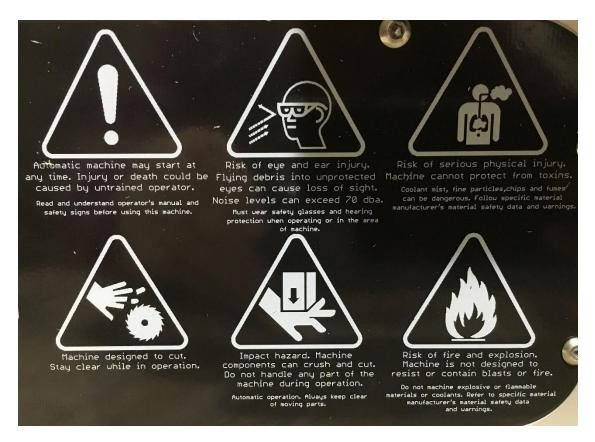
Figure 1 Mill Warning Decal Example
