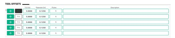
At the far left of each row is the tool measure button. When this button is pressed, the machine will begin the tool measuring process. This includes moving the machine to home followed by bringing the spindle forward and prompting the user to install the proper tool and then press cycle/start. From there the machine will position the tool in front of the tool probe button under the B axis and then finish the probing sequence by pushing the button twice. After the probing
