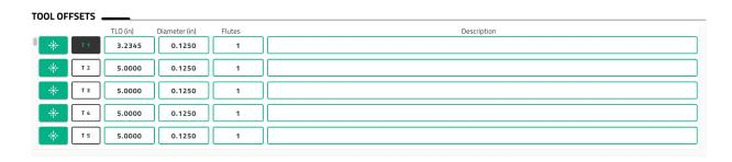
Next to the tool measure button is the active tool indicator and button. This button can be clicked to activate a specific tool number, turning it black. The tool number that is shown as active here should agree with the tool that is listed as active in the far right column of the WORK OFFSETS section discussed earlier.
