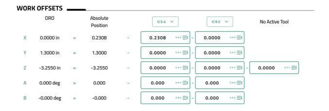
The G92 drop down menu allows users to Zero the DRO in relation to the G92 offsets as well as clear, suspend or restore G92 offsets. The editable fields below this drop down menu function the same as the ones to their left. Using G92 offsets is not as common as G5x offsets and a thorough understanding of how they work should be obtained before attempting to use them.
