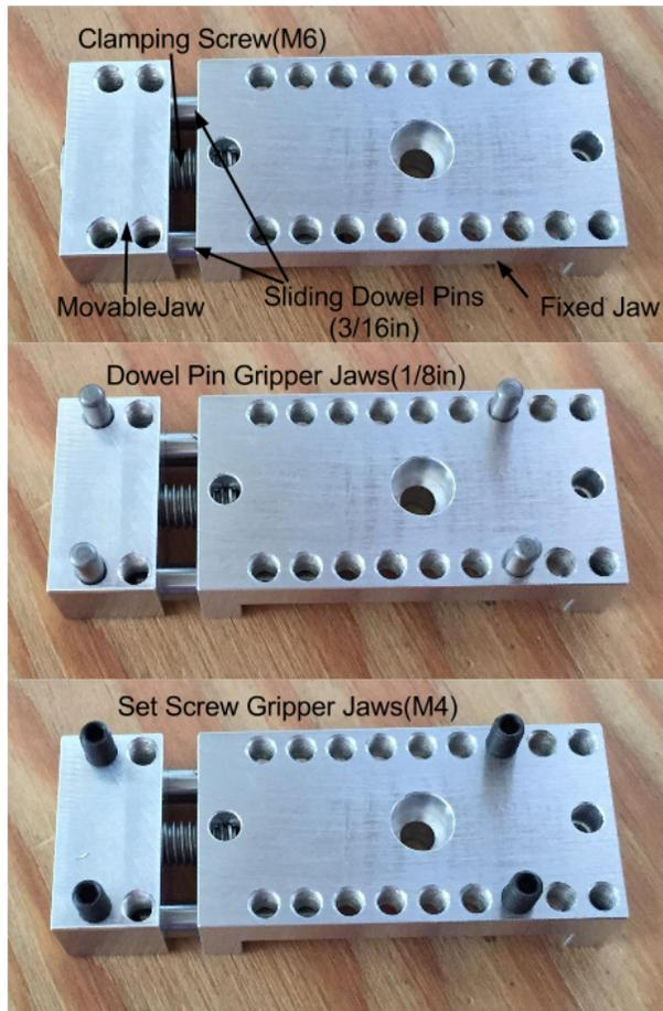
Mounting the vise to the PocketNC V2 mill requires an adapter to bridge the hole in the center of the B-table.
