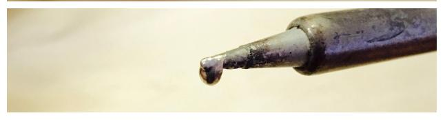
The most effective method for soldering assemblies together will be to apply solder to the iron rather than to the assembly. Once the iron has a sufficient amount of solder on the tip it can be applied to a flux coated copper strip.
