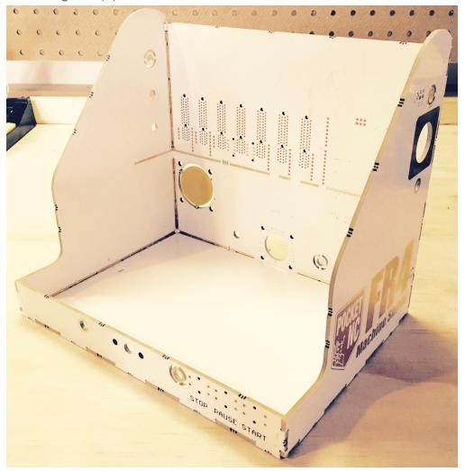
When complete, the main structure should look like the picture above, held together by 6 beads of solder, one in each corner.
