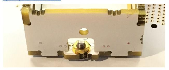
Once the Z assembly has been tacked together install and solder 2 M3 brass nuts (P/N FH001) on the pad shown in the previous photo. Once the brass nuts are soldered in place, finish soldering all joints of the Z assembly and the X assembly.
