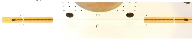
Make sure all components fit together smoothly and without air gaps before soldering. Only two components need to be checked at a time to verify fit. **Note that individual components are soldered together along a copper strip shown in the picture above.**
